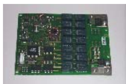
ID ISC.DAT -- automatic tuning circuitry which is installed in each antenne ID ISC.ANT800/600-DA.
